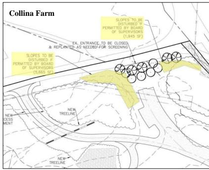
Slopes proposed for disturbance for the Clifton Inn expansion are shown on the inset to the left above and are 369 square feet on non-contiguous slopes. The applicant indicates these have likely been disturbed for internal access roads. The disturbance of the slopes would allow for siting of new guest rooms in a manner that would be secondary to historic structures.
