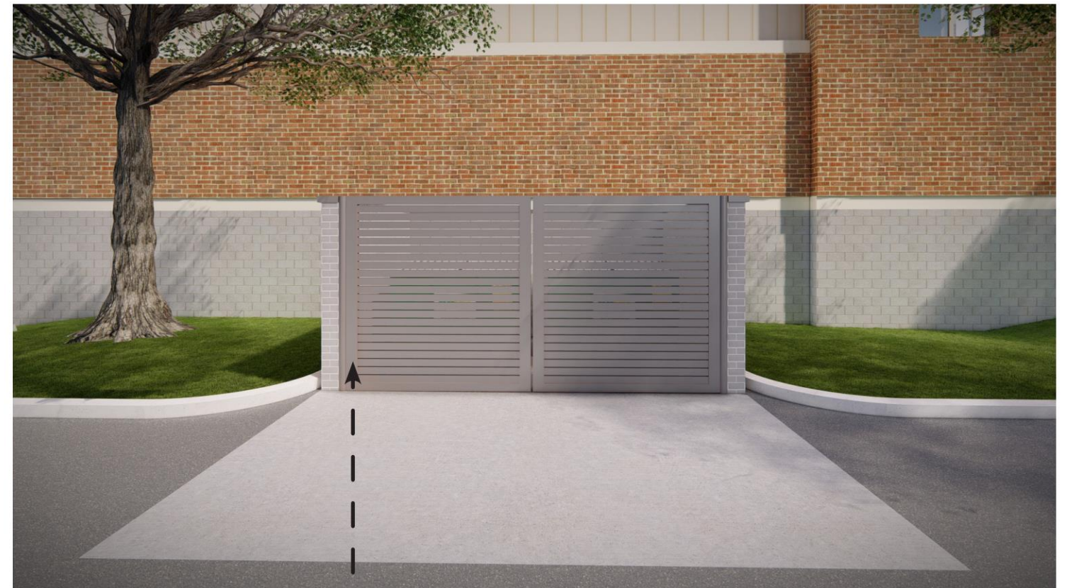
HORIZONTAL, COMPOSITE BOARD DOORS TO BE PAINTED SHERWIN WILLIAMS 9175 "DEEP FOREST BROWN" TO MATCH BUILDING TRIM AND INSTALLED ON STEEL POST HINGES.
