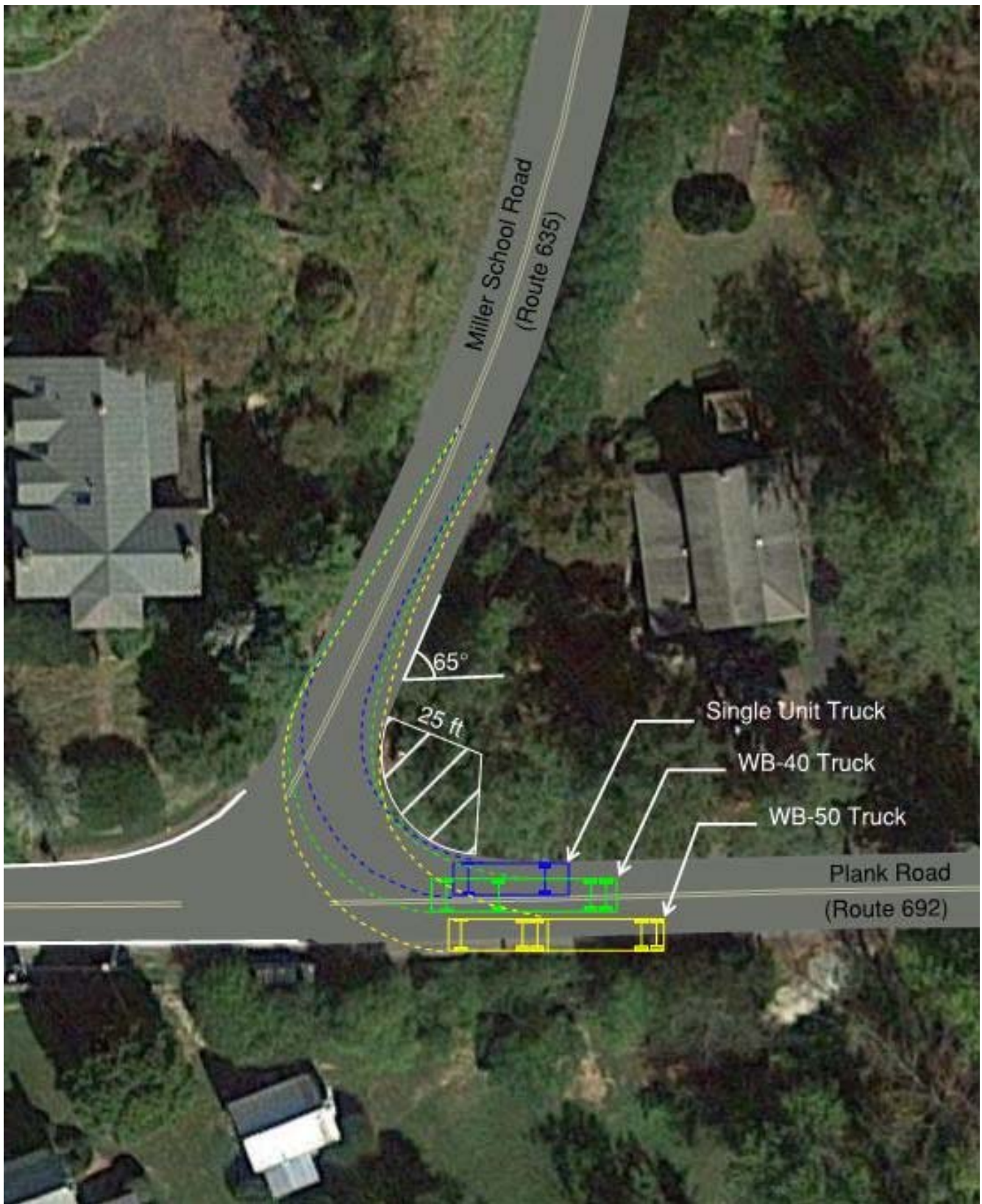
Figure 6: Turning Paths for Single Unit Trucks (30-foot wheelbase), WB-40 Trucks and WB-50 Trucks
