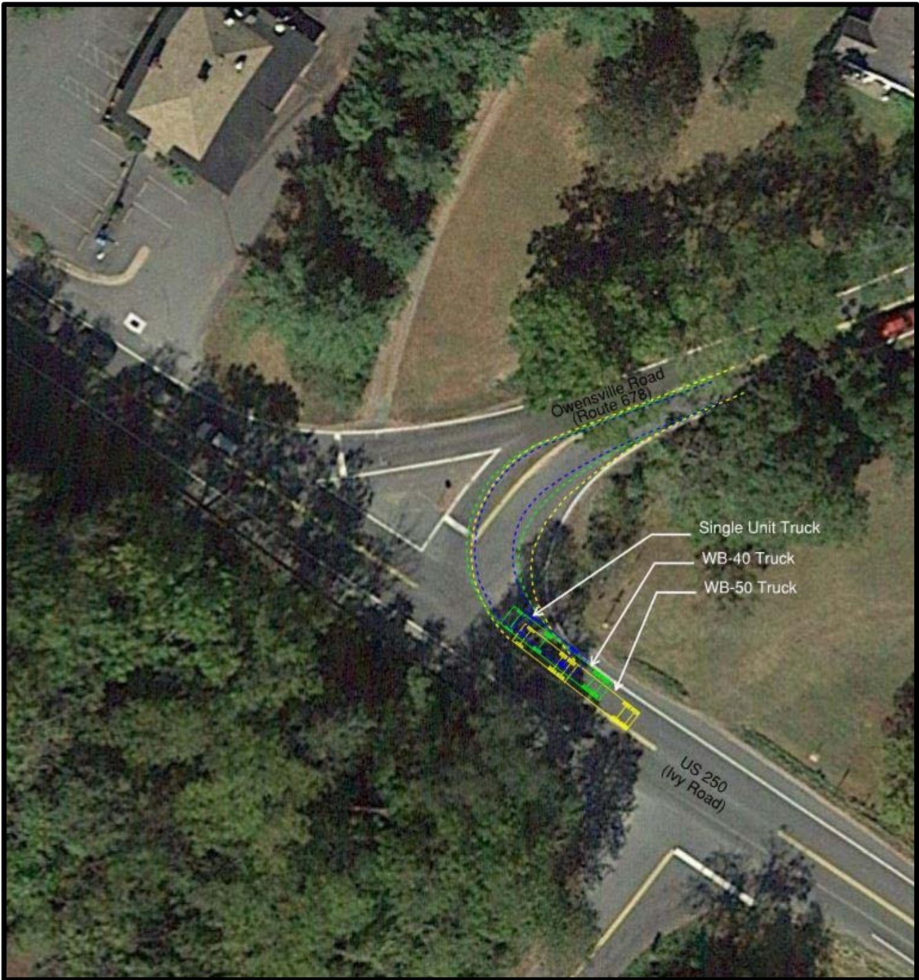
Figure 5: Turning Paths for Single Unit Trucks (30-foot wheelbase), WB-40 Trucks and WB-50 Trucks
