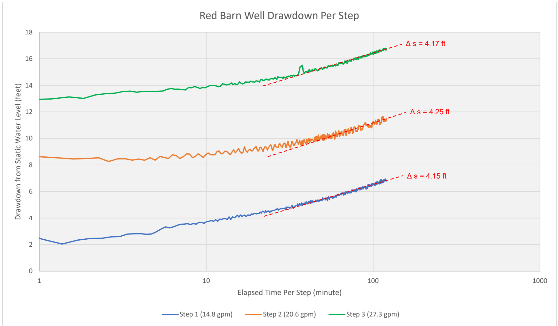
Graph B-2: Red Barn Well step-drawdown pumping test data on a per step basis. The test was performed prior to the well's casing modification and deepening in April 2023.
