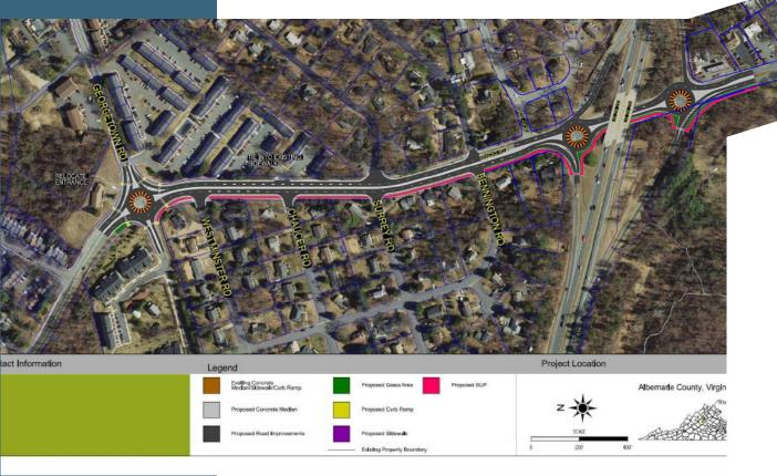
Description: VDOT study to evaluate improvements on Barracks Road to address pedestrian, bike, and transit accessibility and safety and congestion. Recommends roundabouts at Georgetown and bypass ramp termini and shared-use path on the south side of Barracks.
