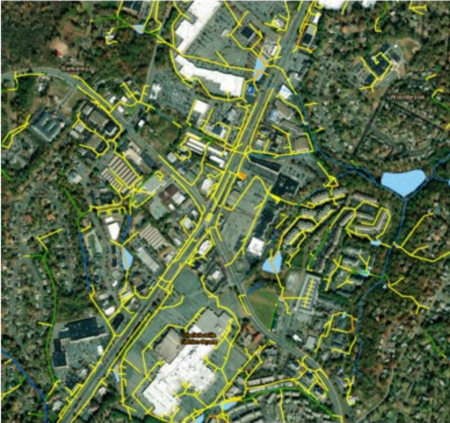
Underground drainage system in the US29 Rio-Hydraulic Road area
