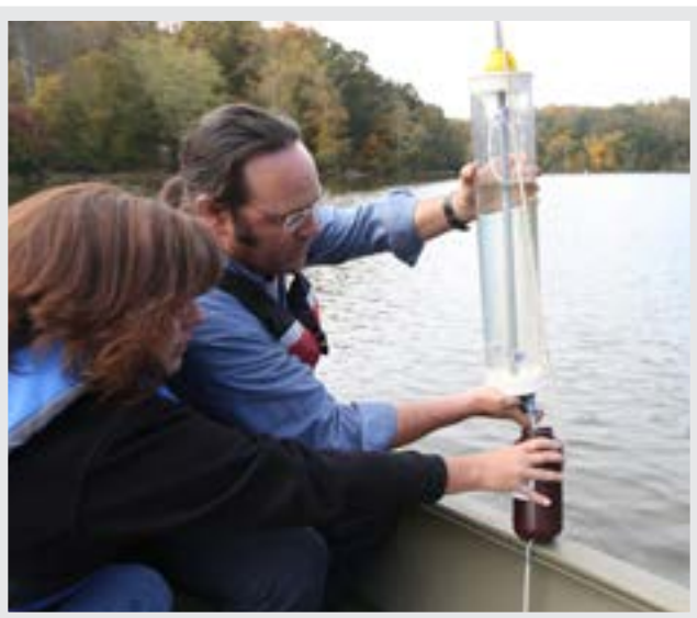
Putting water from Kemmerer sampler into pre-labeled bottle
