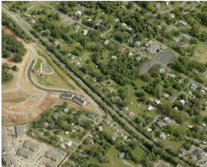
This is an aerial image of the portion of St. George Avenue with a waterway that exists without a vegetated and established stream buffer.
