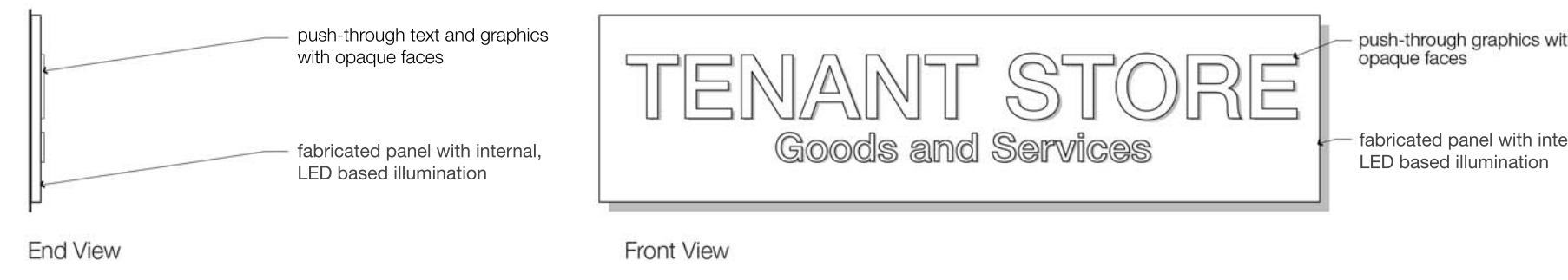
3 Panel Sign w/ Push-Through Text and Graphics SCALE: None
