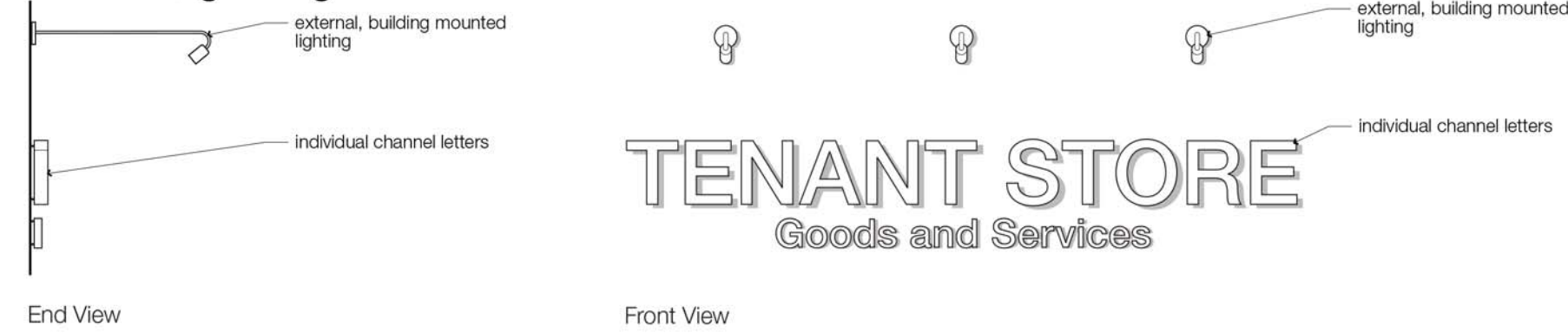
1 Channel Letters w/ External Illumination SCALE: None
