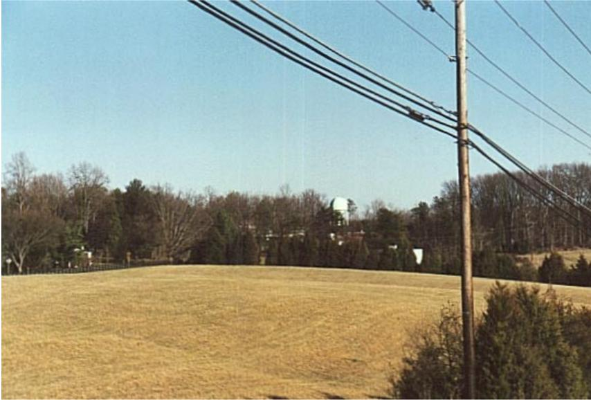
Structures that puncture low ridgelines are ideal platforms for personal wireless service facilities. An example is this Albemarle County Service Authority Water Tank in Crozet. The antennas can be located on the top or sides of the tank with the equipment cabinets hidden by the vegetation.
